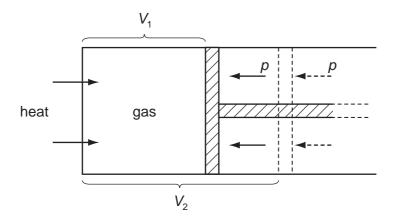
Initially, the gas has a volume  $V_1$  and is in equilibrium with an external pressure p. The gas is then heated slowly so that it expands, pushing the piston back until the volume of the gas has increased to  $V_2$ .
