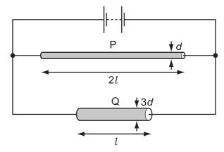
What is the ratio  $\frac{\text{current in P}}{\text{current in Q}}$ ?
